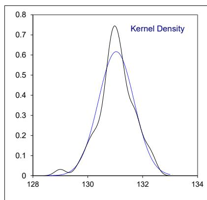
Determination of Kinematic Viscosity at 100°C on sample #21075; results in mm<sup>2</sup>/s
