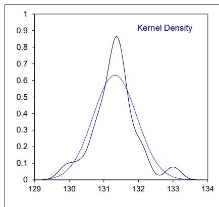
Determination of Kinematic Viscosity Stabinger at 100°C on sample #21075; results in mm<sup>2</sup>/s
