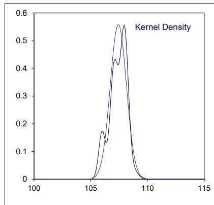
Determination of Kinematic Viscosity Stabinger at 40°C on sample #21075; results in mm<sup>2</sup>/s
